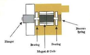
From this picture the plunger can be seen to be mounted on a shaft that passes through two bearings and is held in place by the pressure spring. On the shaft of the plunger is a ferrite core which is affected by magnetism. Around this ferrite core is two coil arrangements. The coil arrangements are made up of two copper wires wrapped around a bobin in both directions and termindated to the electrical connector.
